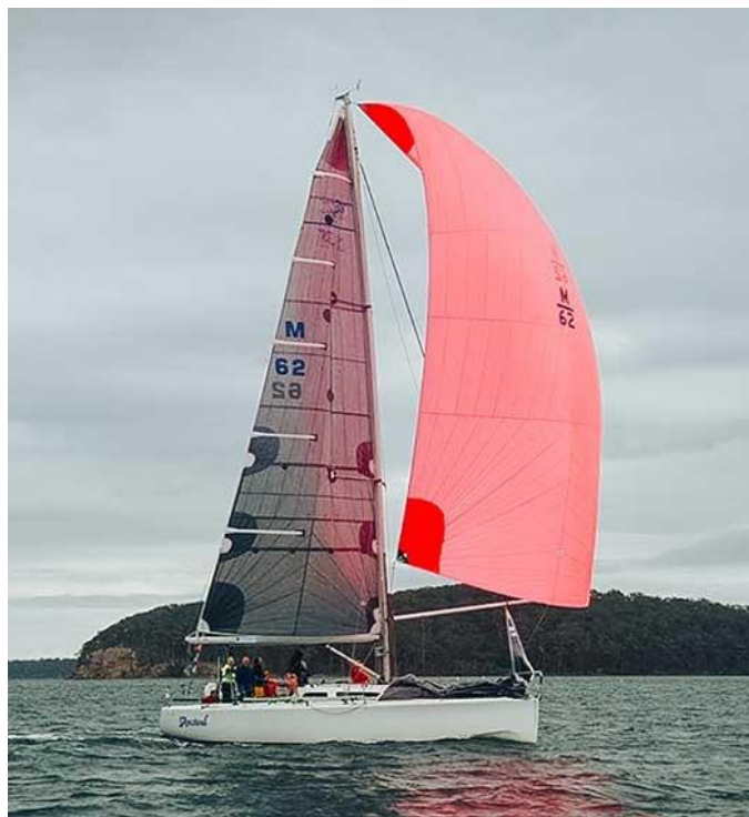
Figure 26: Example of a symmetric spinnaker.
