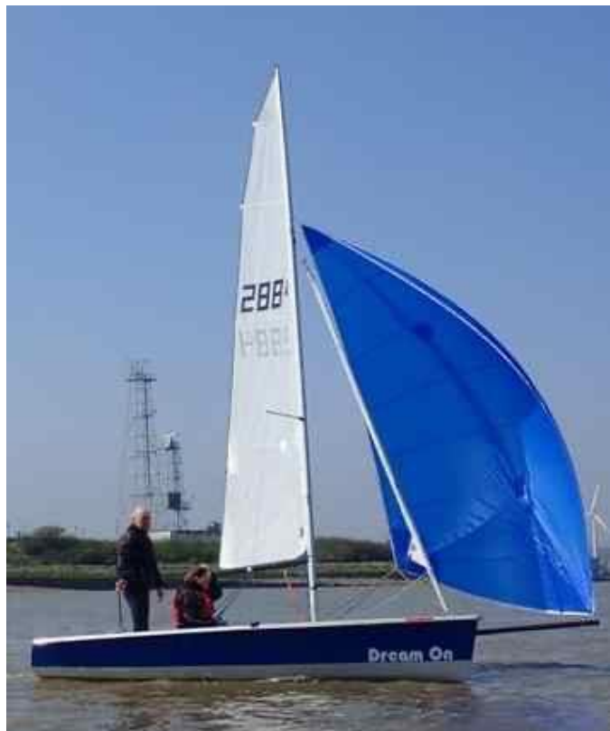
Figure 27: Example of an asymmetric spinnaker.
