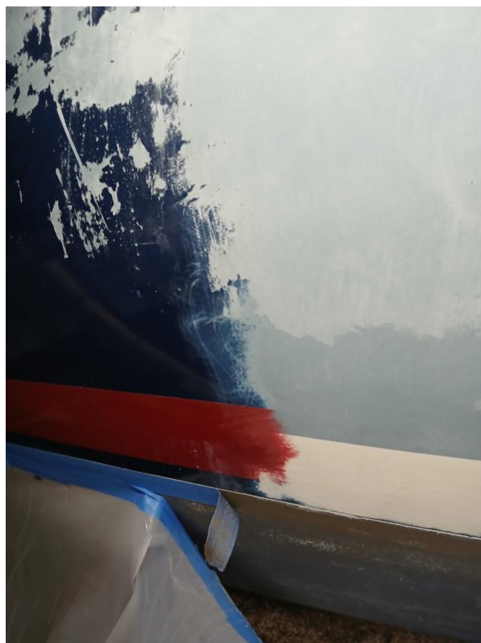
Figure 23: Topside dark blue and red boot stripe, partially stripped, reveals the original light blue-grey topside and white toe rail gelcoat.
