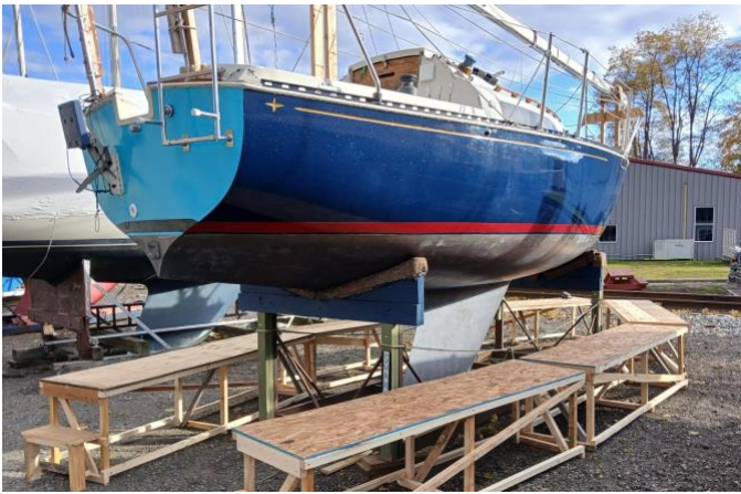
Figure 17: Decals removed and risers built.
