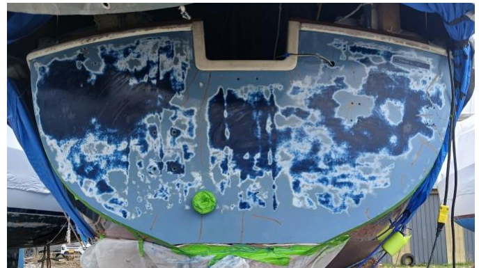
Figure 5: It took a couple sessions of sanding and to fully remove the paint. The light bluish gray is the original gelcoat.
