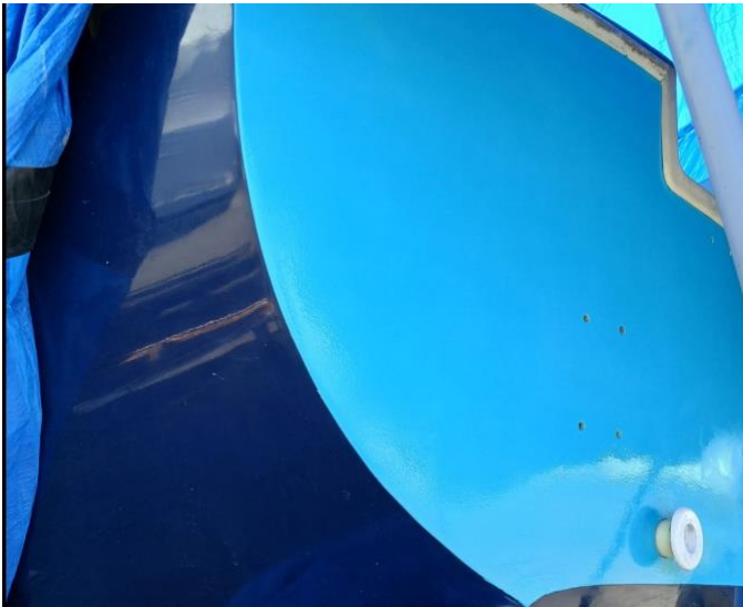
Figure 6: The finished transom sans hardware.
