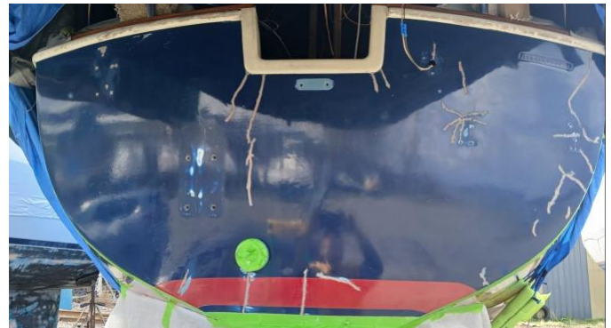
Figure 4: Cracks ground out and filled.
