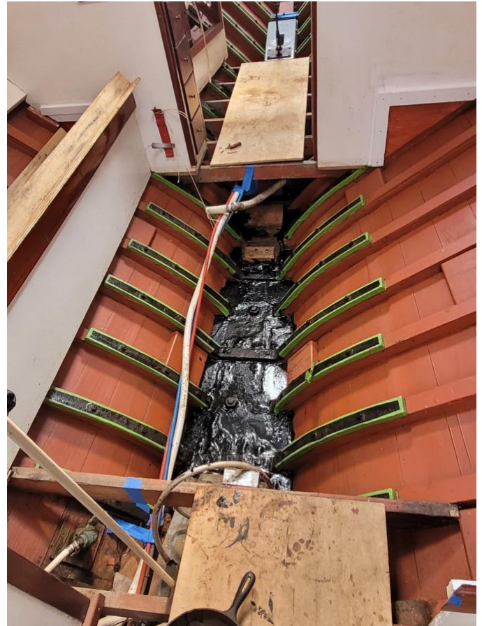
Figure 2: Hull interior painted and tarred, ready for the water tanks.
