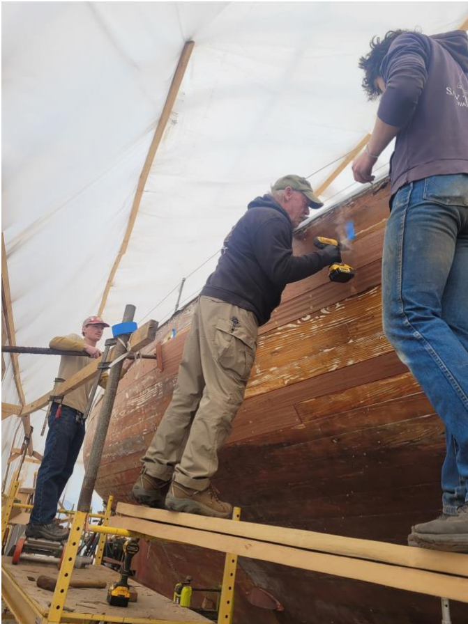
Figure 1: True Love crew work at replacing planking.
