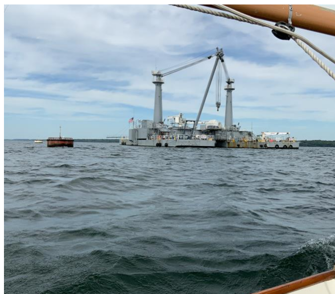
Figure 1: US Navy acoustics research barge, off Dresden, NY, in the center of Seneca Lake. The barge is designed for sonar testing and calibration. Cranes can lift whole sections of ships and it's got its own 2MW generating station. This image from the 2022 race.
