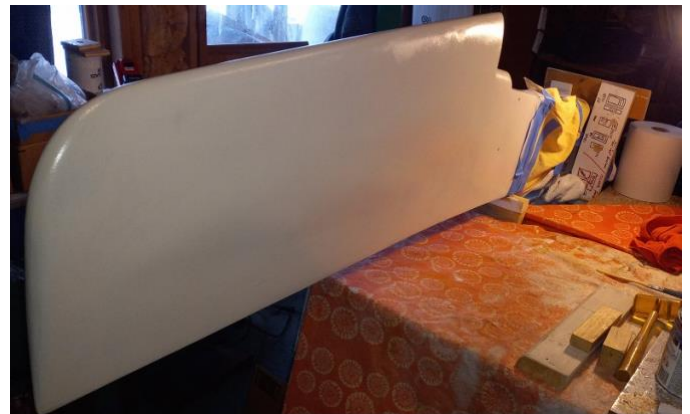
Figure 7: Below the waterline with a couple coats of barrier paint.
