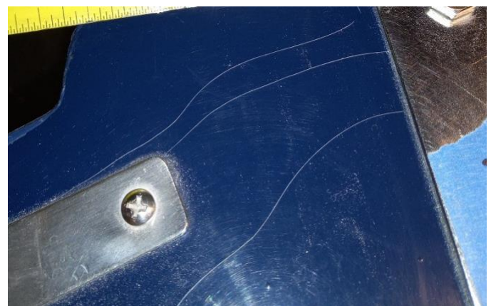
Figure 4: And the cracks on the topside paint.
