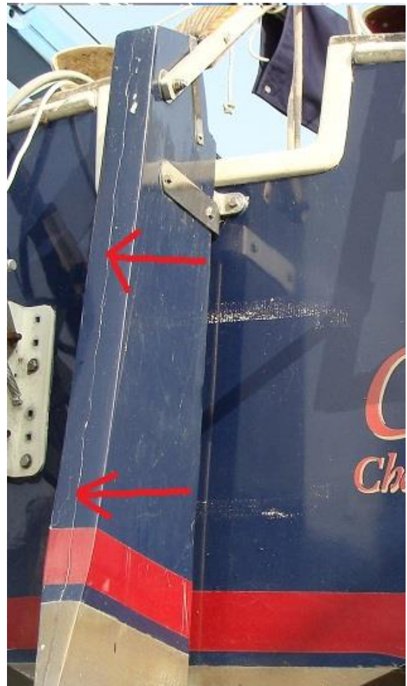
Figure 3: This is what I started with as seen from aft, showing the cracking along the spine.
