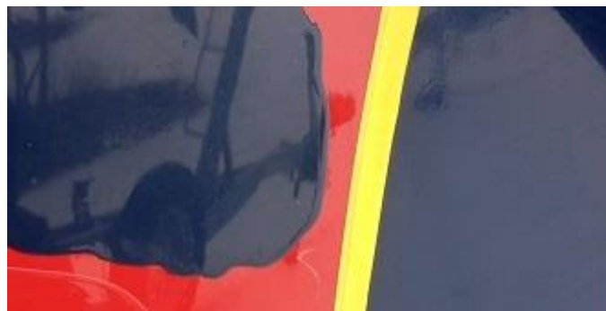
Figure 9: Paint color match. The sample (the dark blue splotch on red on left) against the hull topsides on the right. Notice the reflection in the gloss of the paint. The photo is representative, but to the eye it was a near perfect match.
