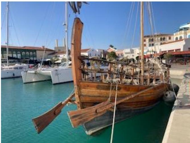
Figure 1: Starboard aft showing canoe end and steering boards. Modern sculpture on stern prow not original, but still cute.
