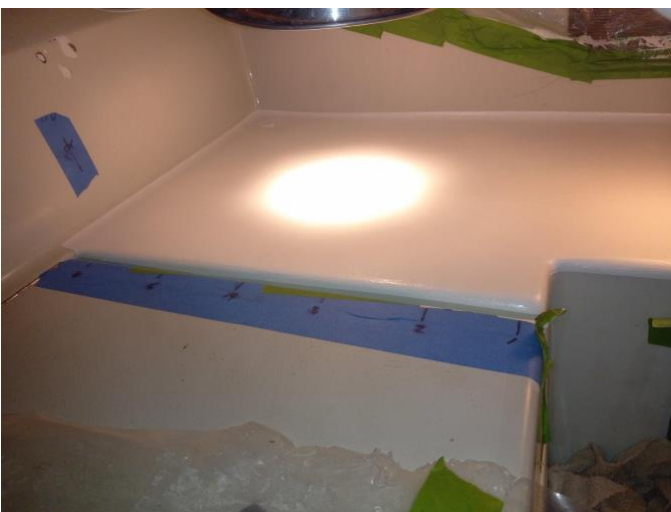
Figure 5: Port side after wet sanding.
