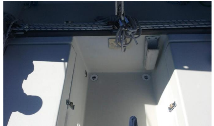
Figure 1: Not a great photo but shown is how the traveler is mounted on the aft end of the bridge deck, forward of the lazarette seats.
