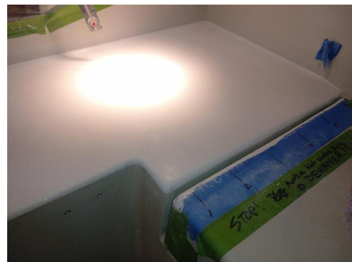
Figure 6: Starboard side after wet sanding.
