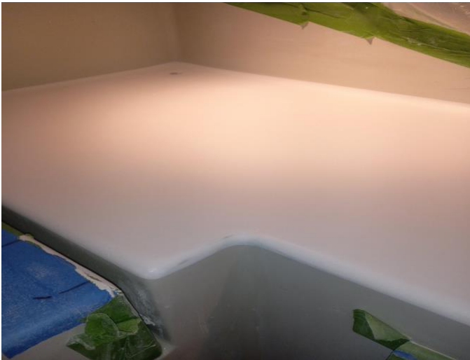
Figure 3: Port side after gel coat cure but before sanding.
