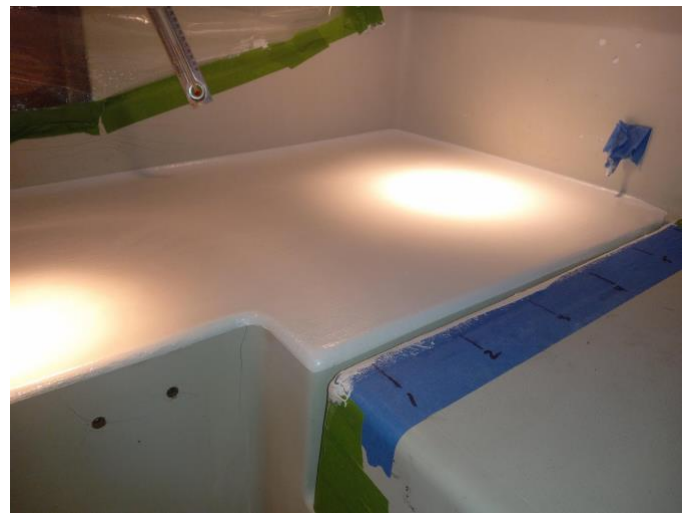
Figure 4: Starboard side after gel coat cure but before sanding.
