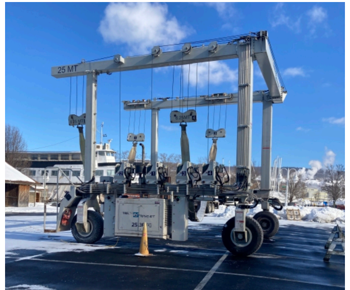
Photo 7: View of the right side of the lift. Note that each set of blocks has its own winch, making it easier to level boats.
