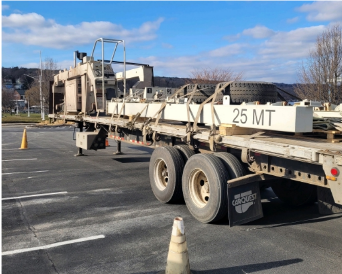
Photo 4: Delivery of the WGV's new travelift. This one is rated for 25 metric tons, or about 55,000 lbs.
