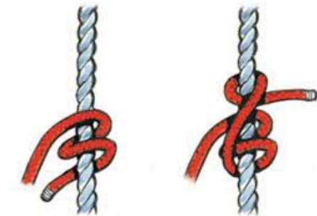
Figure 1: How to tie a rolling hitch.
