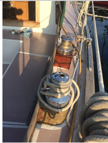
Photo 13: Another view of new pedestals and winches in operating position.
