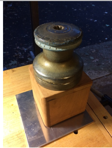
Photo 10: New winch pedestal with all components stacked together.
