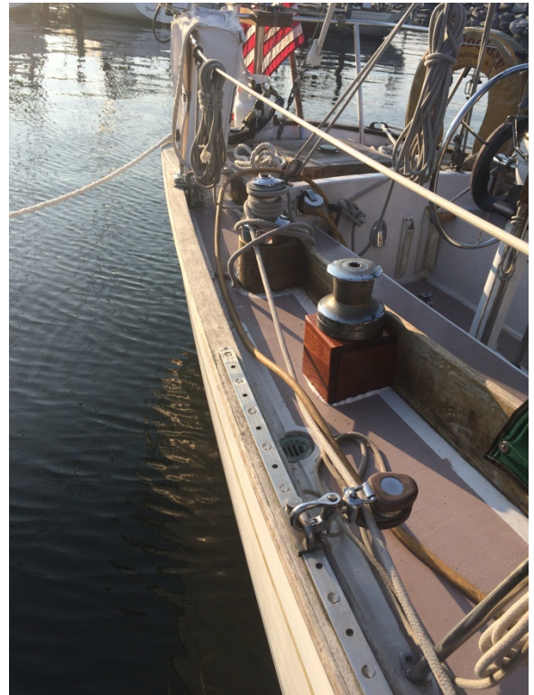
Photo 14: Looking aft toward the new pedestals and winches.
