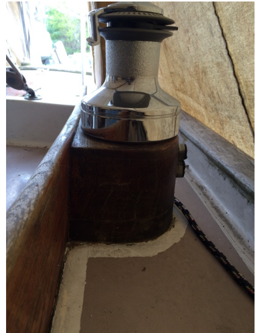
Photo 2: Pedestal mount for existing winches.
