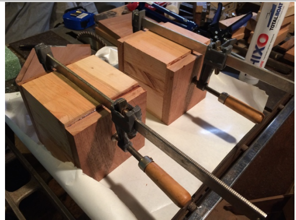
Photo 6: Laminating blocks to create new pedestals.
