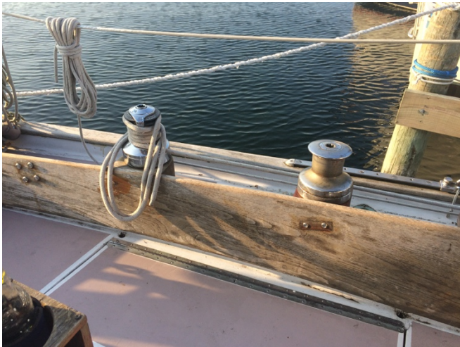
Photo 12: New pedestals and winches mounted and ready for use.
