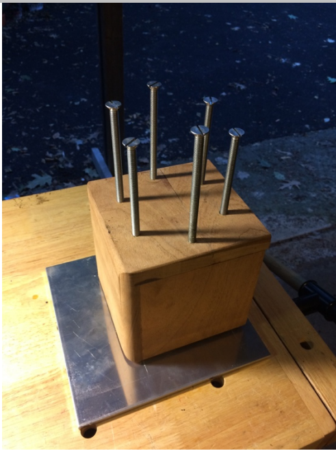
Photo 8: Laminated pedestal with bolts in pre-drilled holes.
