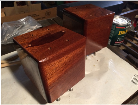
Photo 11: Winch pedestals with three of seven coats of varnish applied.
