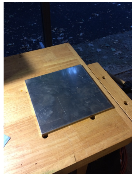
Photo 7: Plate of 1/4-inch aluminum for backer.
