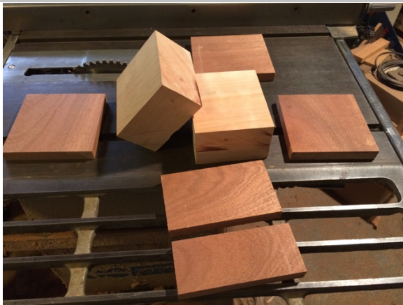
Photo 3: Wood blocks used to laminate up new pedestals.
