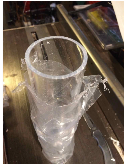
Photo 1: 2-inch acrylic tubing used as a container for the desiccant. It was cut on a table saw. This shot shows the edges after being deburred.
