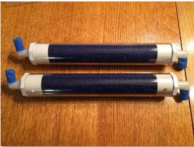
Photo 10: Completed moisture trap tubes filled with desiccant beads. Ends are taped off to minimize air exchange in order to keep the desiccant fresh until it is installed in the boat.
