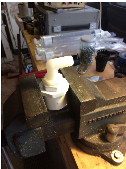
Photo 3: Assembled end cap for the acrylic tubing.
