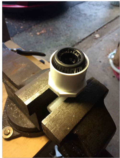
Photo 9: The strainer is simply press-fit into the end cap. Desiccant beads will hold it in place.
