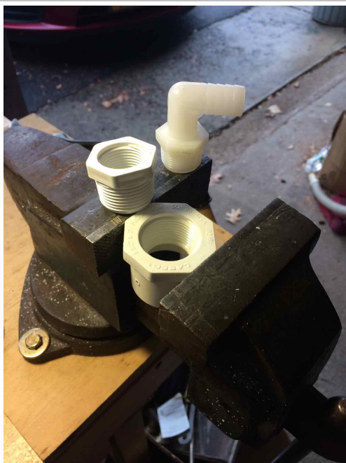
Photo 2: Assembling the end caps for the acrylic tubing. This picture shows the components used to reduce down from the 2-inch tubing to a 5/8-inch hose barb.
