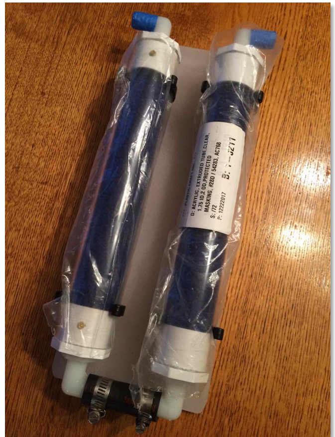
Photo 12: Completely assembled fuel vent moisture trap. The two containers are plumbed in series so that one can be removed at a time for recharging. The plastic wrap is there to protect the acrylic tubing during installation as acrylic scratches easily.
