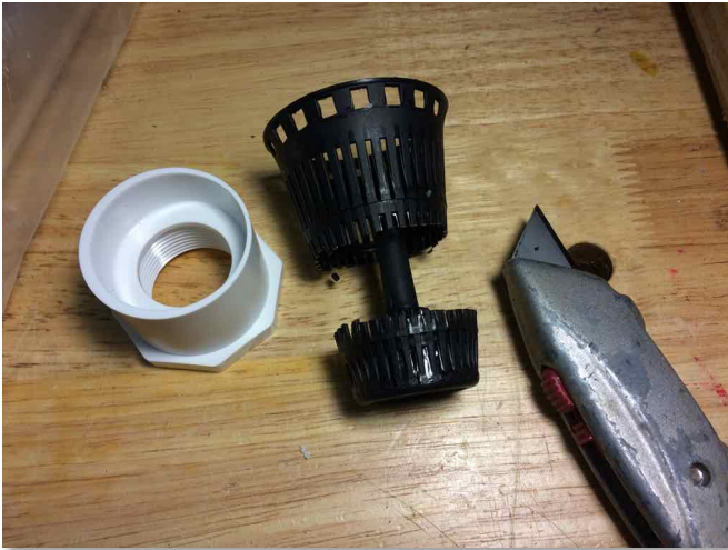
Photo 7: Strainer trimmed to the correct diameter to fit into the end cap.
