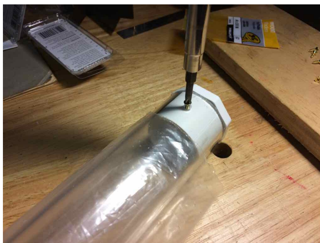
Photo 5: Attaching small screws to hold the end caps in place. Care must be taken as acrylic will crack easily.
