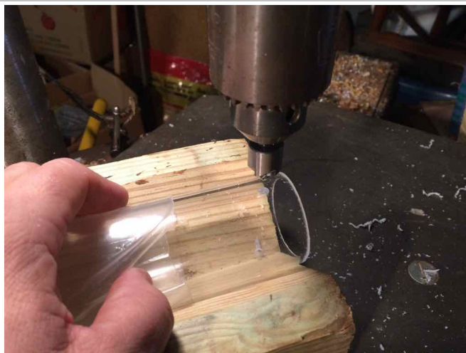
Photo 4: Drilling and countersinking holes in the acrylic tubing for screws that will hold the end caps in place. Care must be taken as acrylic cracks easily.
