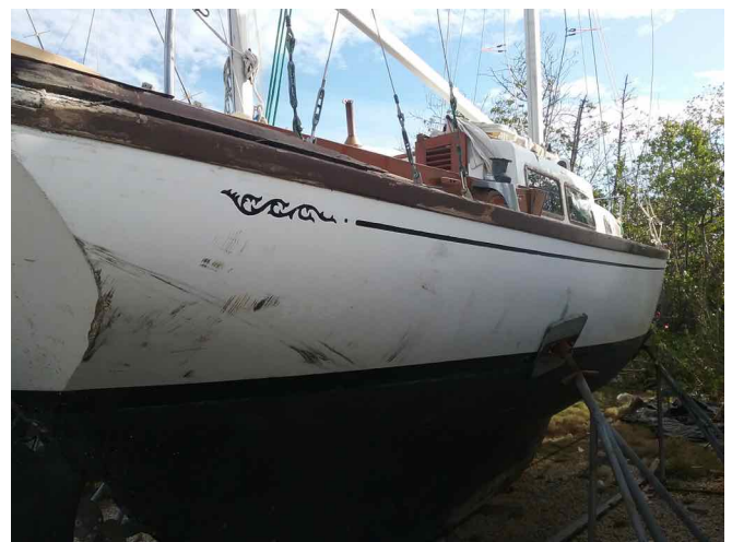
Photo 2: Some of Contessa's injuries: Broken port lights, damaged gunwale, and various scrapes and bruises on her starboard side.
