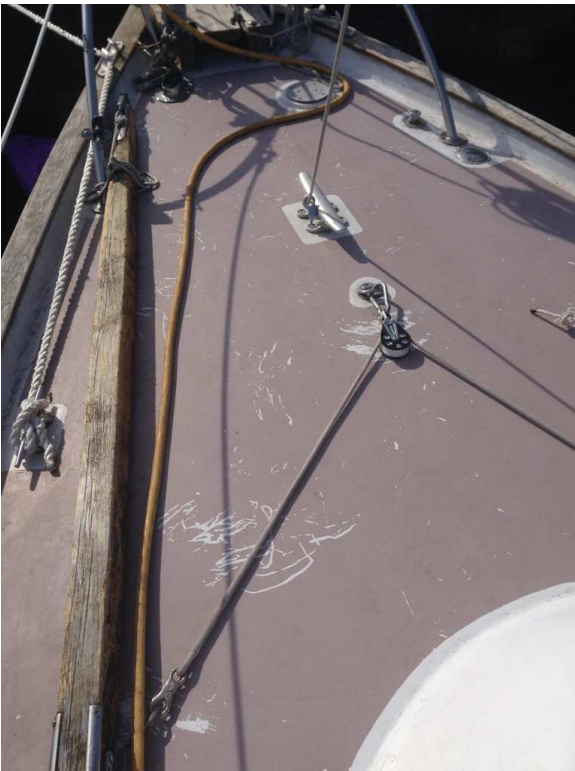
Photo 8 - Tomfoolery 's foredeck showing gouges left by the furler as it flogged in the wind following the failure.
