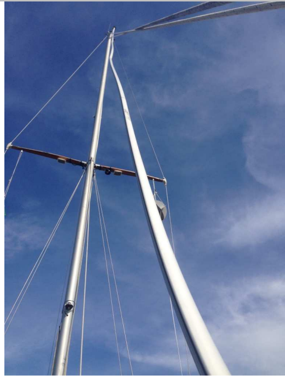
Photo 5 - Tomfoolery's not-so-straight furler extrusion after the foresail had been removed.
