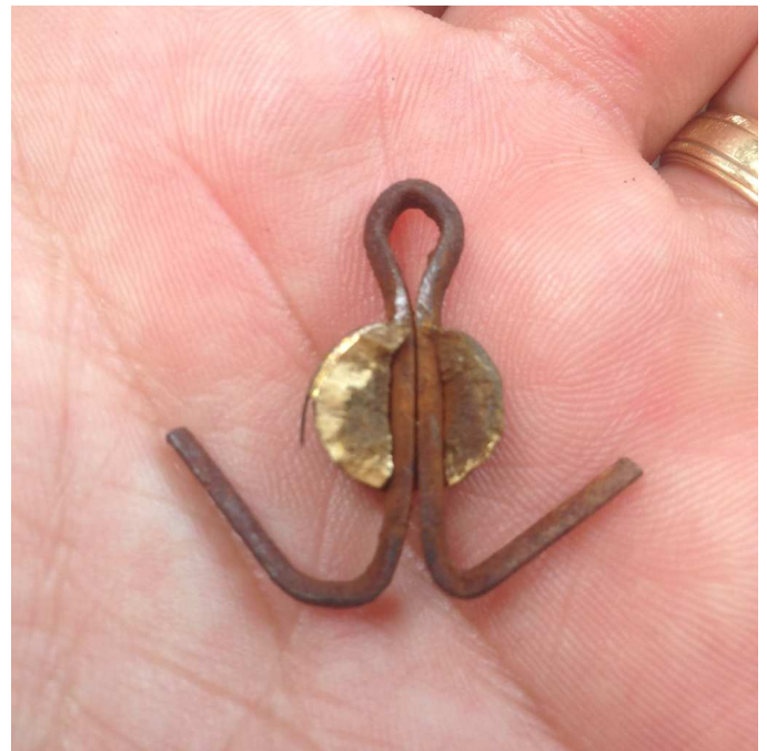
Photo 9 - Portion of the lower forestay clevis pin found on Tomfoolery 's foredeck during cleanup.
