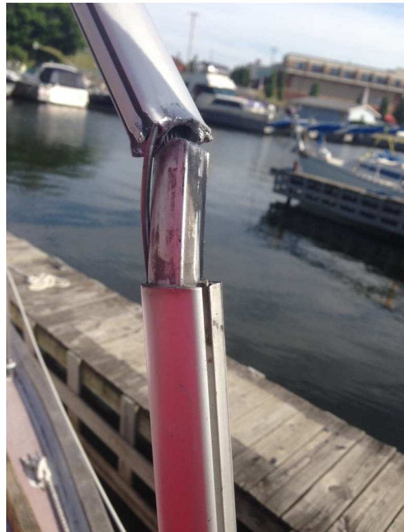
Photo 6 - Sheared joint on Tomfoolery's furler.
