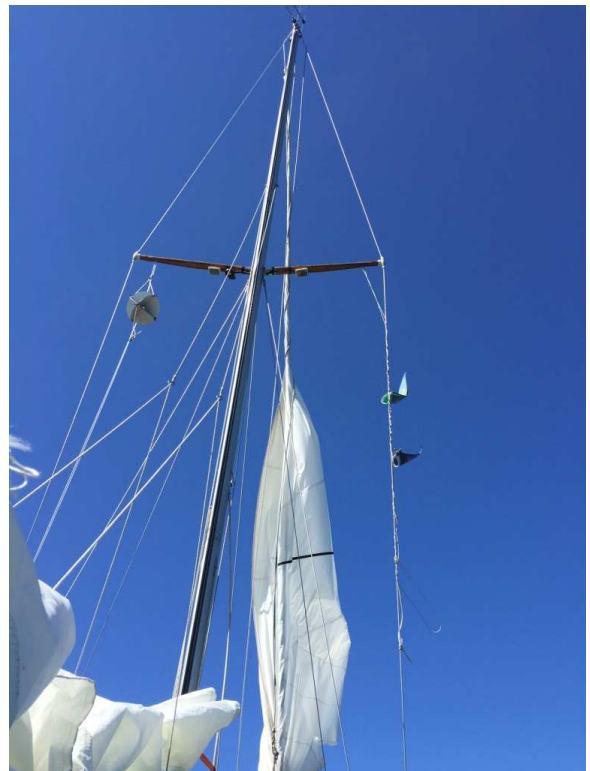
Photos 3-4 - Deck-level view of Tomfoolery's jury rig as they limp back to harbor.
