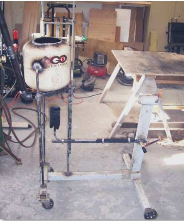
Figure 11 - Homemade cauldron for casting lead.
