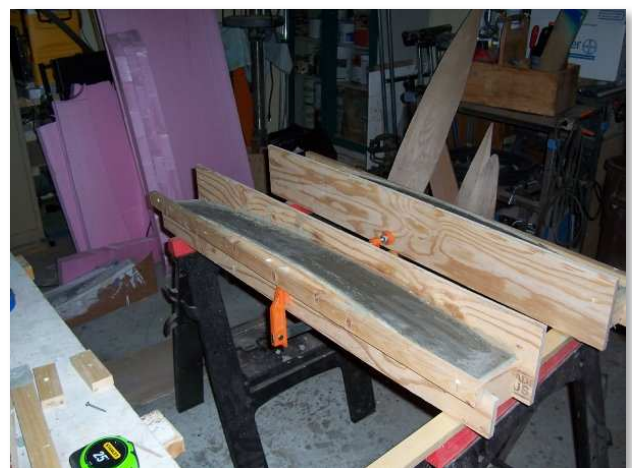
Figure 6 - Resulting positive keel forms.
