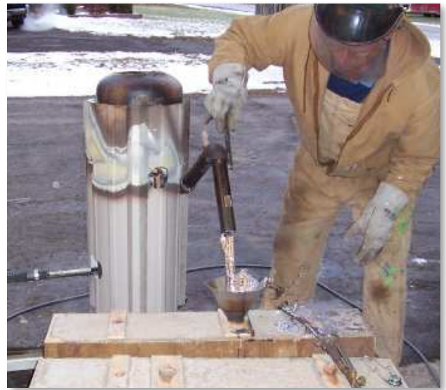
Figure 14 - Once the lead was melted all that I had to do was lower the pipe to direct the lead into the mold.
