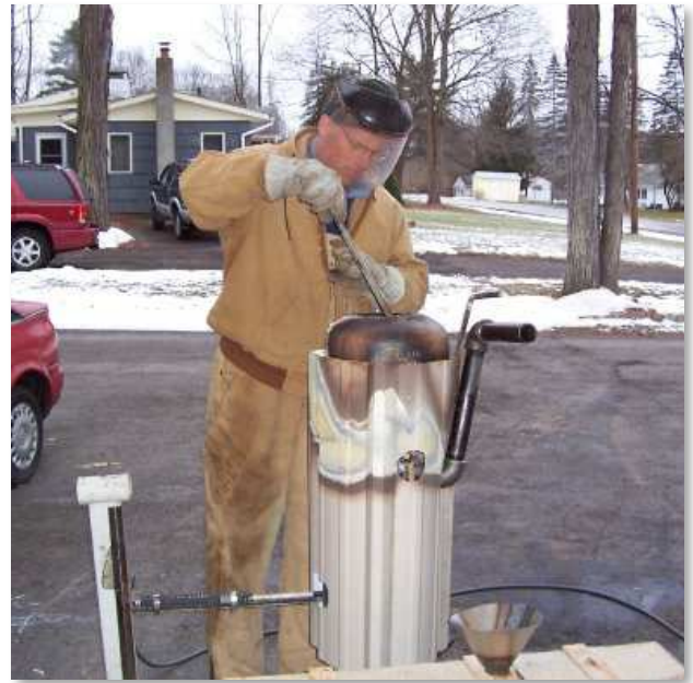
Figure 13 - Checking the molten lead prior to the pour.
