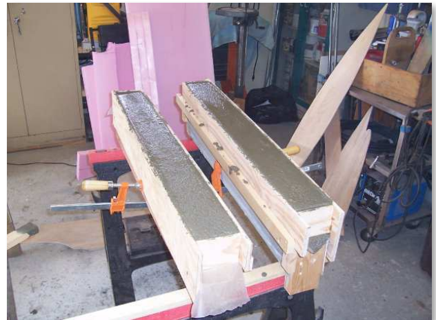
Figure 5 - Making positive forms from the keel castings.
