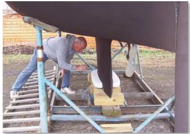
Figure 9 – Test fitting of the plaster prototypes.
