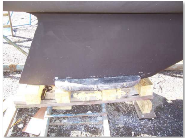
Figure 18 - Keel bulbs following attachment.
