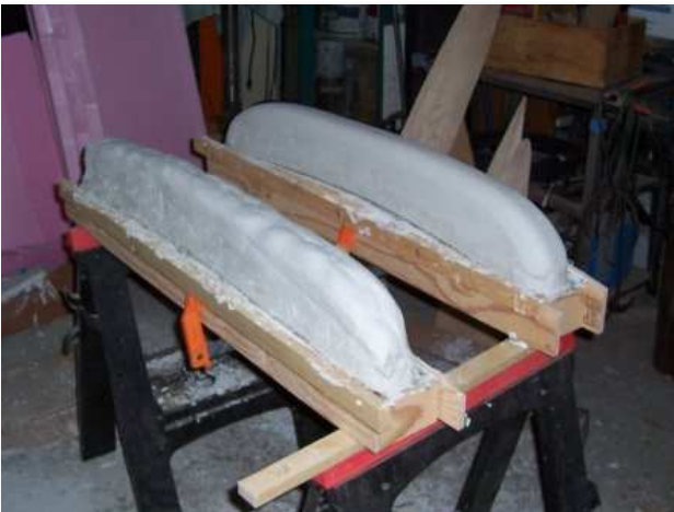
Figure 8 – Plaster prototypes before and after sanding.
