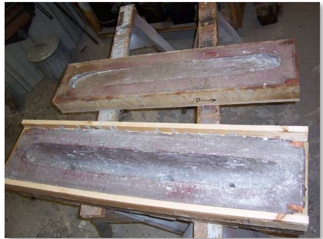
Figure 10 – Casting molds. It doesn't show well in the picture, but I also incorporated recesses for the mounting bolts.
