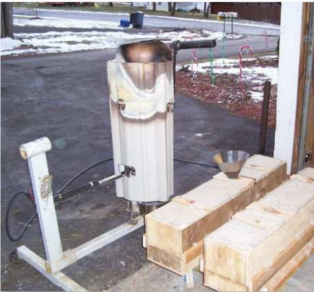
Figure 12 - Casting furnace in action. Note funnel in the mold for the pour.
