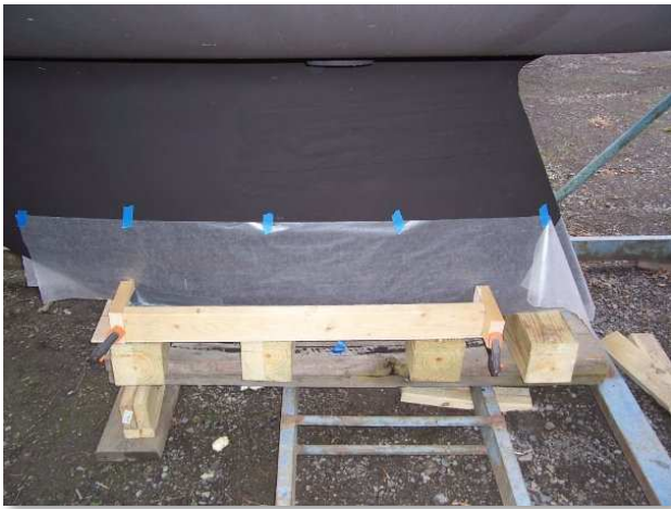
Figure 2 - The 6 x 6 blocks are cut in half diagonally to form a wedge which made them removable.
