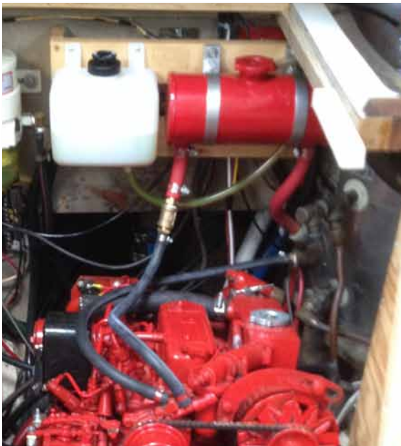
Location of new coolant accumulator and expansion tank.
