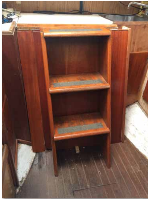
Cabinetry modifications after application of mahogany veneer and varnish.
