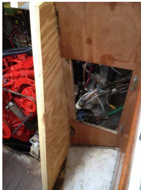
Cabinetry modifications to accommodate the new moter, which is slightly larger and has accessories in different locations.
