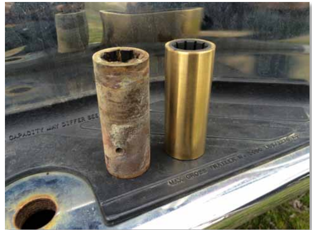
New and old cutlass bearings in a side-by-side comparison. You can see the wear in the rubber flutes in the old bearing.
