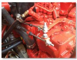
would not fit in the space provided and also limited the amount of movement in the control cable itself. As a result, I wound up fabricating my own terminations out of small brass strips and stainless steel hardware. (Fortunately, I'm in fresh water where I can get away with using brass. Long term, stainless steel is probably a better choice.) By using the strips, I was able to utilize the factory mount points for the cables without modification.
