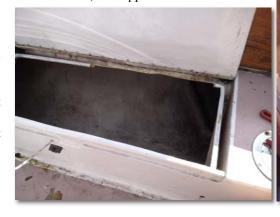
required to remove a lip in the opening through which we could then easily pass the tank. The good news is that the lip is easily glassed back in and will not result in cosmetic damage to the exterior of the boat.
