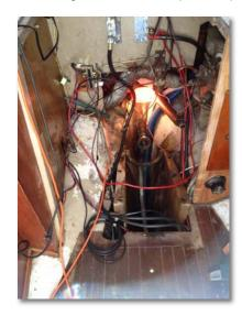
fired up and we used multiple loads of hot water and detergent to break down the grease and oil in the engine compartment. After scrubbing the worst of the dirt away, some time was spent cleaning up the wiring in the compartment. Since rewiring will be a future project for this boat, no attempt was made to get everything "just perfect".
