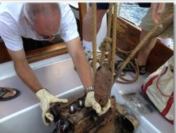
ionway. The next phase of the lift then put through the companionwhere we pushed the load out onto the bridge The deck. final part of the lift moved the engine from the bridge deck to cockpit the sole.
