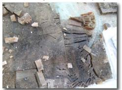
looks like. What you can't see is that many of these balsa tiles have delaminated from the fiberglass and are no longer attached to anything.
